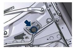
The brake pads wear could cause the fluid level to fall. However, low fluid
