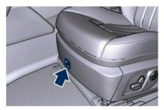
Press the switch downward to move the pedals forward (toward the front of the vehicle).
