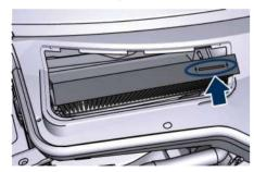
Close the filter access cover and reinstall the access door.
