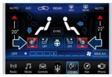
Within 15 seconds, touch the driver or passenger seat soft-key a second time to select LO-level heating.
