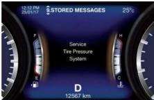
• Once you repair, replace or reinstall a tire with the compact spare tire, the TPMS will update automatically. The TPMS light (!) will turn OFF and the graphic in the instrument cluster will display a new pressure value instead of dashes (--), as long as no tire pressure is below the lowpressure warning limit in any of the four tires. The vehicle may need to be driven for up to 20 minutes above 24 km/h (15 mph) in order for the TPMS to acquire and process the updated information.
