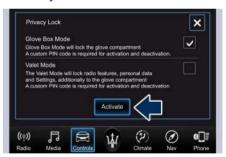
Using the keypad, enter the four digits of the PIN and touch "OK". The system prompts you re-enter the PIN code to confirm it.
