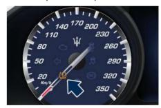
To reactivate the TPMS, replace all four wheel and tire assemblies (road tires) with tires endowed with TPMS sensors.
