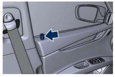
To unlock the front doors, pull the inside door handle to the first detent.
