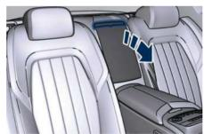
Behind the reclining shelf, you may access a power source of 12 V and a USB high capacity port for charging portable devices.
