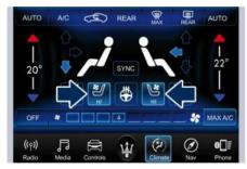
Within 15 seconds, touch the driver or passenger seat soft-key a second time to select LO-level ventilation.
