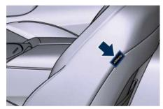
When the air bag deploys, it opens the seam between the front and side of the seat's trim cover. Each air bag deploys independently; a left side impact deploys the left air bag only and a right side impact deploys the right air bag only.
