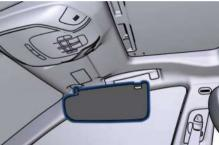
By lowering the visor you can access the courtesy mirror with incorporated light illuminating automatically (with the ignition switch in **RUN**) by raising the mirror protective cover. Before raising the visor, close the mirror cover.
