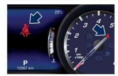
The BeltAlert® warning sequence begins after the vehicle speed is over 8 km/h (5 mph) for more than 19 seconds, by blinking the seat belt reminder light 🔏 and by sounding an intermittent chime.
