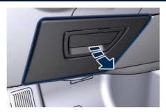
The compartment is ca. 25-30 cm (10-12 in) deep and is lit by two courtesy lights when open (the light automatically switches off when the compartment is closed).
