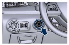
The Keyless Ignition Node (KIN) has three operating setups indicated on the outer ring. Pressing and releasing the middle button, you can switch from one setup to the next without starting the engine, the switched on indication will turn amber.
