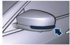
The external mirrors can be equipped also with approach and courtesy LEDs, lighting up when the vehicle entry/exit lights are activated.
