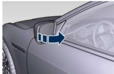
Press the switch once and the mirrors will fold in; press the switch a second time to reset the mirrors to the standard position.
