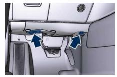
• The ventilation of the lower part of the rear passengers compartment is made by means of fixed vents positioned under the front seats and they are specific for dual-zone and four-zone A/C system.
