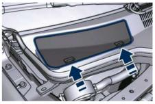
Unsnap both ends and lift the filter access cover.
