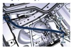
• If a refilling is necessary: unscrew the filler neck cap.
