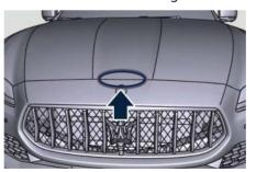
• Slightly lift the hood and push the safety catch as indicated by the arrow. The safety catch is located in the center of the lid.
