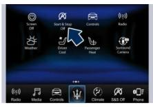
To quickly disable the Start&Stop function, you can insert it in the main menu bar, at the bottom of the MTC+ display, as follows:
