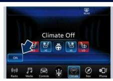
The "OFF" soft-key will appear in place of "ON" when the A/C is on. If the A/C system has been turned off, temperature values in the upper status bar will be obscured in all MTC+ modes.
