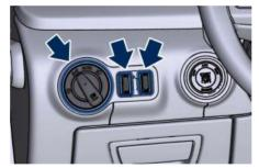
Rotate the light switch to the **305** or to the **30** position: the instrument cluster will display the related telltale.
