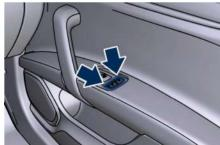
If the vehicle has been locked from inside with the above figured switches, the fuel filler flap remains unlocked.
