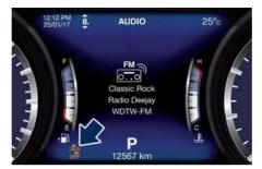
This warning light informs the driver that FCW is disabled. This warning light will light even when the activation of another driver assistance feature or drive mode (example: \$\bar{z}\$ (ESC Off) disables the FCW.
