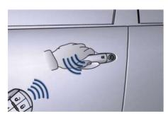
• If the unlock command is enabled by pressing the specific dutton on the key fob RKE transmitter or by the Passive Entry system, the "illuminated entry" mode will activate. Courtesy
