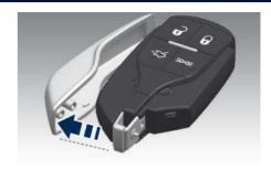
Separate both parts of the key fob case.
