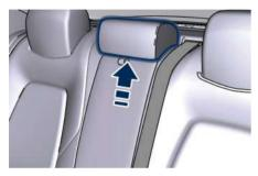
To lower the head restraint, press the push button, located at the foot of the head restraint on the left side, and push downward on the head restraint.
