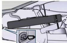
When the seatback is folded to the upright position, make sure it is latched by strongly pulling on the top of the seatback above the seat strap.
