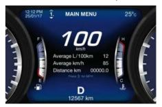
Further to speed, the main area can indicate three lines that can be set to the same options and in the top right or top left area. When these three lines are present and turn-by-turn navigation is on, main menu area will automatically show navigation information. For further details, please refer to "Maserati Touch Control Plus (MTC+)" quide.
