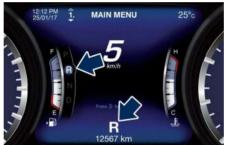
If the vehicle is in D (Drive) status, in M +/- (Manual) or temporarily in manual drive mode, the gear position is indicated beside the lever status ("D" or "M"), on the lower part of the display.
