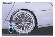
Place the jack near the wheel to be changed as illustrated. Make sure that the head of the jack is correctly inserted in one of the slots 1 or 2 under the longitudinal member.
