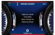
If the driver keeps his/her hands away from the steering wheel (for more than 8 to 10 seconds), also the ACC system is deactivated ( white ACC symbol on the display) and will have to be reset. The aid of LKA system will be disabled as well. In these cases the display will not show the attention level colour anymore and the vehicle will be controlled by the driver only.
