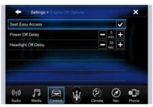
Power Off Delay (Power duration after engine shutdown)
