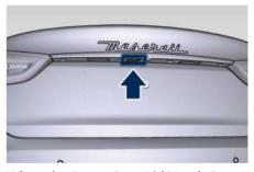
When the Power Boot Lid/Hands Free is open, to move it there are two buttons positioned on its right lower part as indicated in figure.
