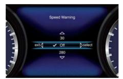
Scroll with the switch in the  $\triangle$  or  $\blacktriangledown$  arrow directions to view the selectable options.
