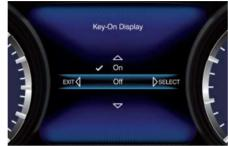
When engine is started and ignition device is pressed to stop it, it is possible to set "Key-Off Display", "On" or "Off" to obtain the following display settings:
