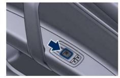
There are single window controls on each passenger door trim panel, which operate the corresponding window. The window controls will operate only when the ignition switch is in the ACC or RUN position.
