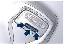
If one or more doors are opened, the front and rear dome lights will turn on for 27 seconds. If the door is closed before this time, the lights will dim and subsequently switch off after about 3 seconds.
