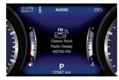
The display will show the audio status (source and current audio track) as set on the MTC+. It is possible to display 5 lines of 15 alphanumeric characters. Displays Audio Statuses are:
