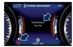
In this case, slow down until temperature returns to normal level (the light will turn off).
