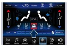
Within 15 seconds, touch the heated steering wheel soft-key a second time to turn it off.
