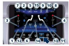
Press any of controls on the climate control panel to display "Climate" screen.
