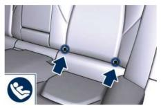
In addition, there are tether strap anchorages behind each rear seat. The anchorages are located in the panel between the rear seatback and the rear window and are under a plastic cover (indicated in the figure) with the anchorage symbol on it.
