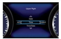
Press and release the switch (▶) to select an item. The notification of setting saved appears as a popup for 2 seconds, then the display will show the last-modified item
