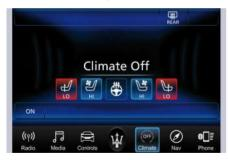
When the MTC+ System is in any mode other than "Climate" ("Radio", "Media", "Controls", etc.) the settings of driver and passenger temperature and air flow distribution will be indicated on the upper part of the
