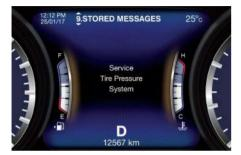
The instrument cluster will also display pressure values in place of the dashes (--). On the next ignition switch cycle the "Service Tire Pressure System" message will no longer be displayed as long as no system fault exists.
