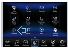
In this mode the MTC+ System allows you to access the following programmable features (some of them are optional or for a specific model/version and may not be available on your vehicle): Display, Units, Voice Commands, Clock, Safety & Driving Assistant, Lights, Doors & Locks, Auto-On Comfort & Remote Start, Engine Off Options, Audio, Phone/Bluetooth, Radio Setup, Restore Settings and Clear Personal Data.
