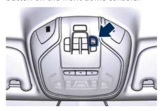
After pressing the button the instrument cluster will display the state of front parking sensors for approximately five seconds. The button LED will be on when the front sensors are disabled. The button LED will be off when the front sensors are enabled. If the button is pressed and the system requires service, the LED will blink momentarily, and then the LED will be on.
