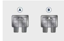
On the vehicle are mainly used with mini-and maxi-fuses with blade engagement.
