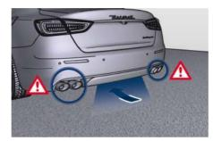
In order for the sensors to detect your foot movement, move your foot towards the vehicle rather than sideways and immediately pull it back: from this moment, the Power Boot Lid/Hands Free will activate within two seconds.
