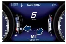
Manual mode can be activated at any time, with no need to release the brake pedal.
