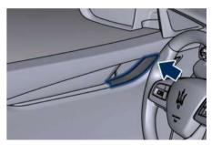
To unlock the rear doors, pull the door lock knob on the door trim panel upward.
