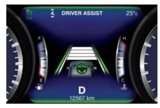
The yellow attention level colour appears when the driver removes his/her hands from the steering wheel for 3 to 5 seconds and the  $\bigcirc$  symbol with the figure of the hands will occupy the whole central area of the display.
