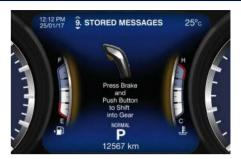
The lever functions like a joystick, so releasing it after giving the command, it automatically returns to the two stable positions (vertical in line with "R", "N" and "D" or in line with "-" and "+" when in "M +/-" mode).
