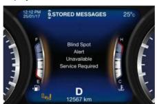
In these cases avoid using the system and have the vehicle inspected at the **Service Network**.
