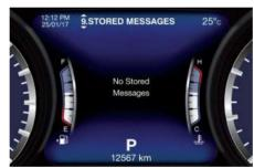
Press and release the switch in the ▲ or ▼ arrow directions to scroll the stored messages.
