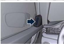
The fixed vents under the dashboard are aimed at ventilating the lower part of the front passenger compartment.
