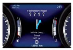
While getting closer to a turn, the sections referred to the distance already travelled will switch off while the ones referred to the distance yet to be travelled will remain on.
