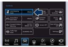
Touching the soft-key on the side the driver can change the setting. Driver warnings can be only "Visual" or "Visual & Haptic" (default mode). System response can be set to "Early", "Medium" (default mode) or "Late". System reaction force can be set to "Low", "Medium" (default mode) or "High".
