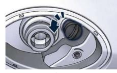
• Insert the end of the cap into the hole of the filler door hinge.
